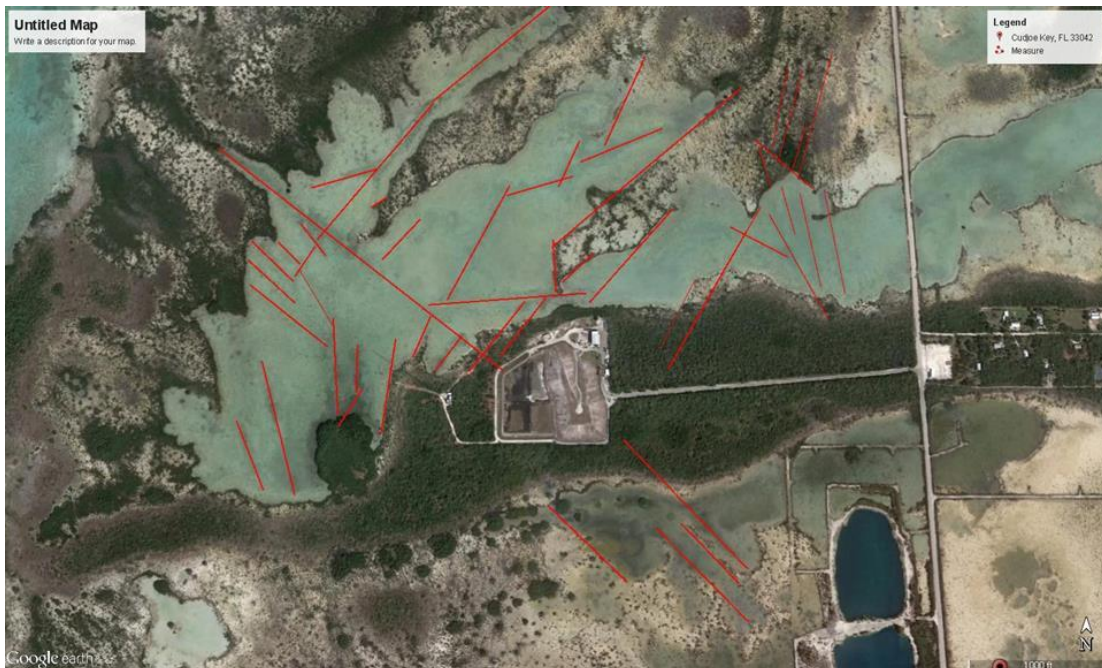
Figure 6: Satellite image (Google) with delineation of linear features (in red) within waterbodies selected for monitoring
