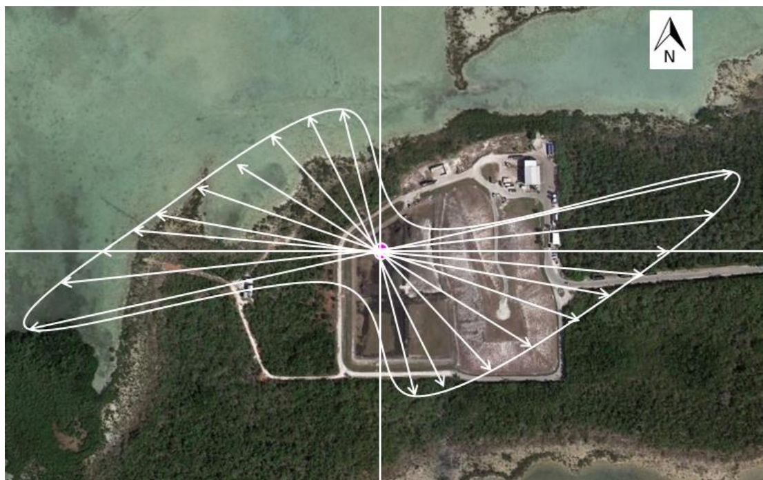
Figure 27: Hypothetical underground flow velocity field for water migrating from injection depth (80 ft to 120 ft) to shallow unconfined aquifer and surface waters.
