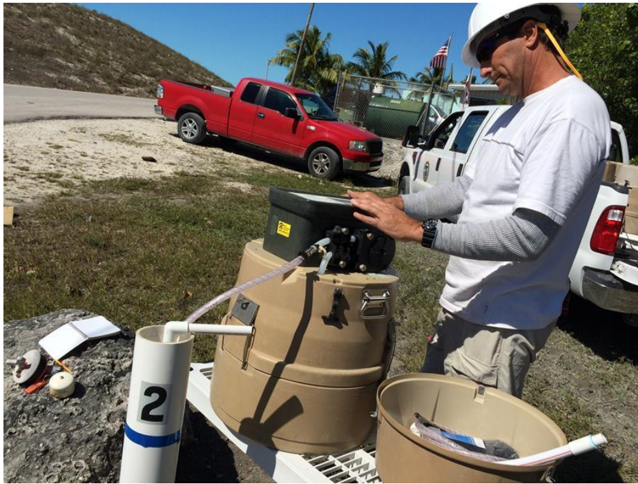
Figure 12: Connecting ISCO Autosampler to OW2
