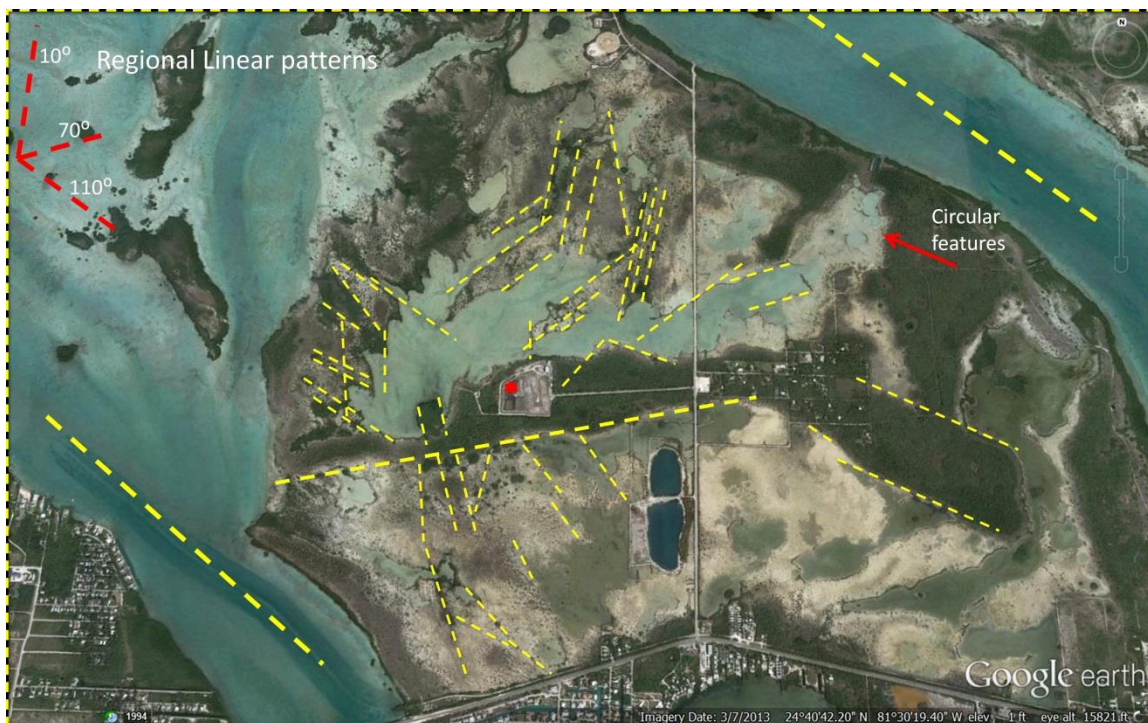
Figure 2: Linear feature map of Cudjoe Key. A significant number of linear features in Cudjoe have similar trend as those identified at regional scale (Lower Keys scale), especially those sets with azimuth 70° and 110° (heavy lines)
