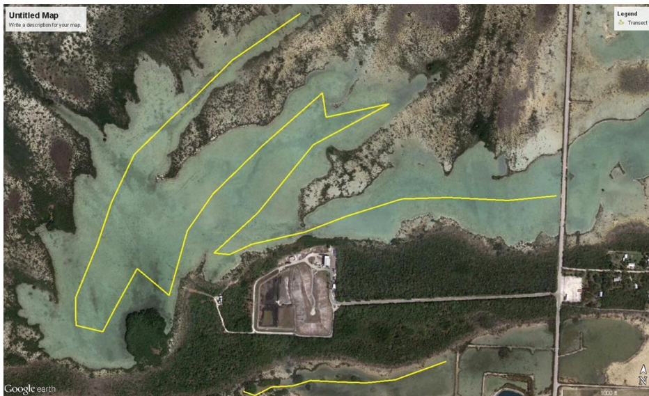
Figure 14: Designed transects for dye and physical-chemical WQ determinations
