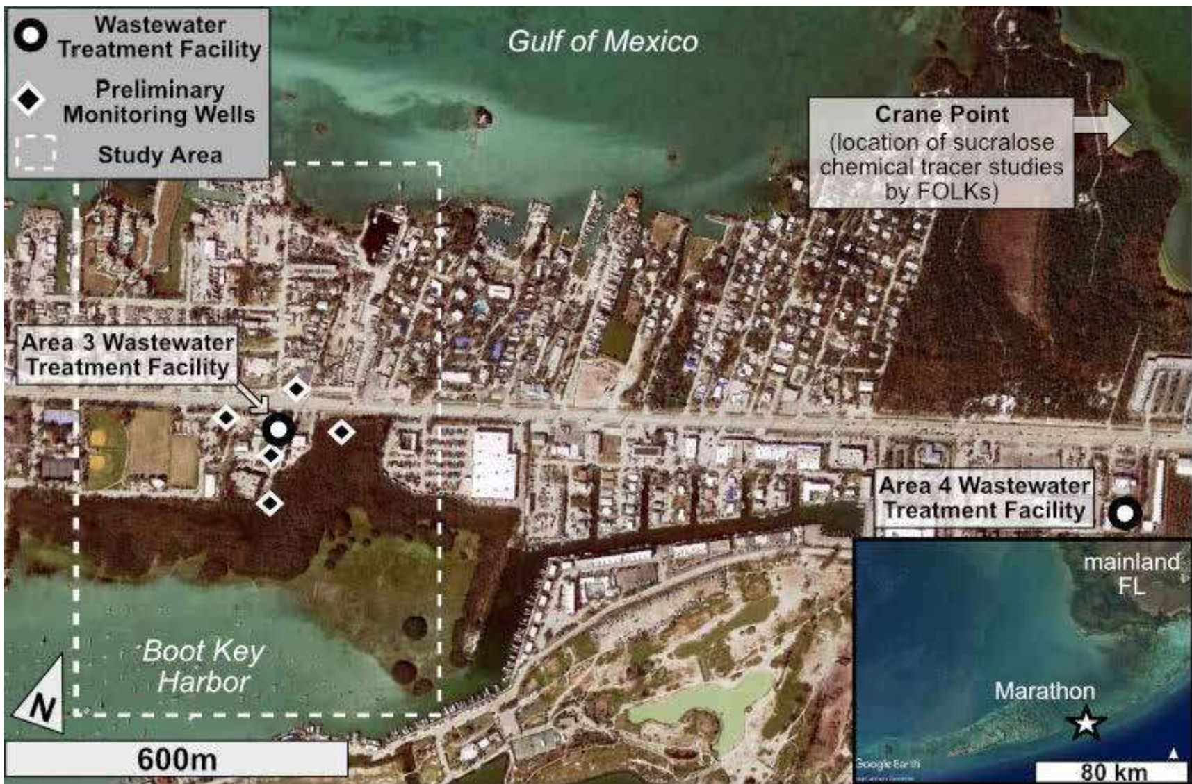
Figure 28: Locations of Monitoring Wells Installed by PSU in 2021
